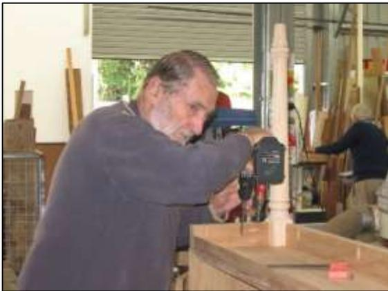
Malcolm can be seen fixing turned legs to Bob's newly completed table using the pocket hole joinery system with pan headed square drive screws.
