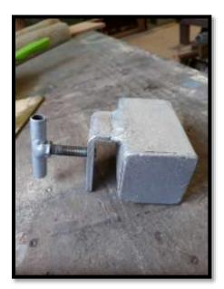
Following a request from our Woodies colleagues for a variable length stop for repeating items such as equal length chair leg blanks on the drop saw, I fabricated the pictured item from various scrap metal pieces.
