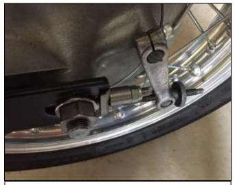
New spacer under the nut of the rear wheel adjuster
