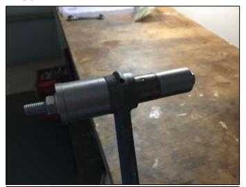
New tool installing the small end bush with a bolt.
